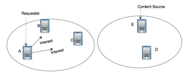
Figure 3.1: Requester and content source in disjoint transmission ranges
