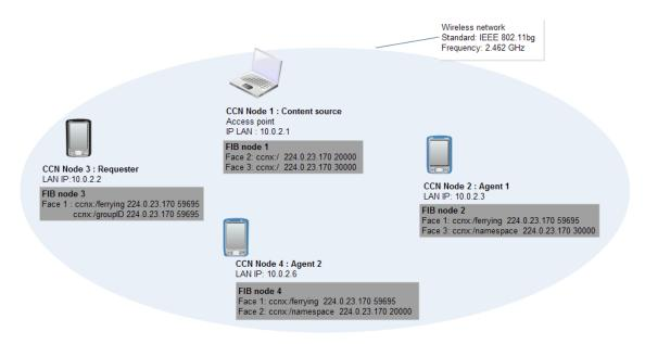
Figure 5.18: FIB configuration of scenario 3.
