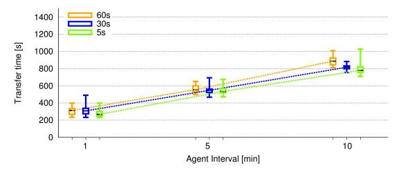
Figure 5.16: Transfer time using different probe intervals with different agent intervals.
