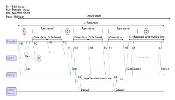
Figure 5.14: Message exchanged during scenario 3: interruption at the first agent.
