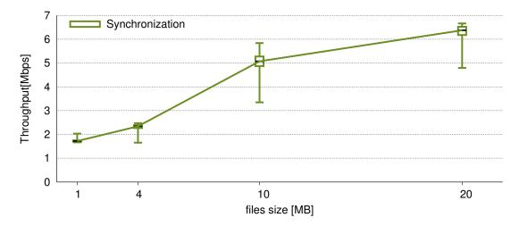
**Figure 5.13:** Throughput of the synchronization mechanism between the home and mobile repositories with different file sizes.
