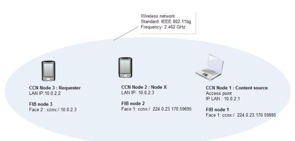
Figure 5.5: Topology used to evaluate congetfile application over two hops.
