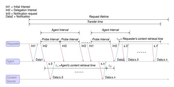
Figure 5.10: Relation between Probe Interval, Agent Interval and transfer time.
