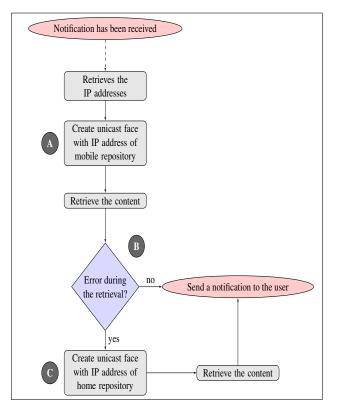
Figure 4.2: Flow chart of the last part of the content retrieval process at the Requester node
