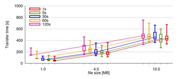
Figure 5.12: Transfer time using different probe intervals with different file sizes.
