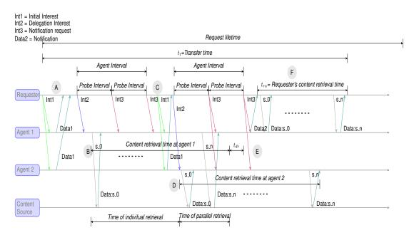
**Figure 5.17:** Message exchanged during scenario 3: parallel content retrievals, probe interval is smaller than agent interval.
