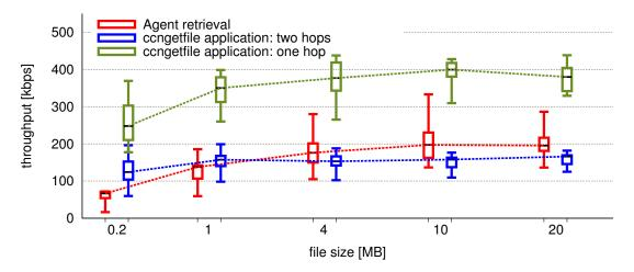
**Figure 5.6:** Throughput of the implemented mechanism compared with congetfile content downloads. The communication is performed via unicast and multicast according to the test setups.
