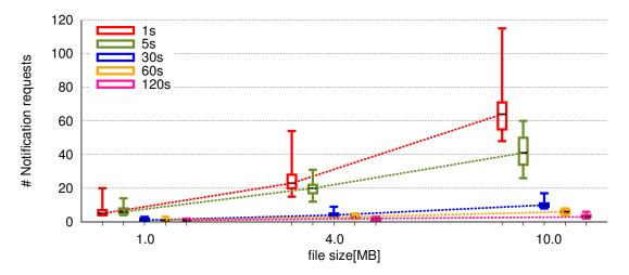
Figure 5.11: Number of notification requests using different probe intervals with different file sizes.
