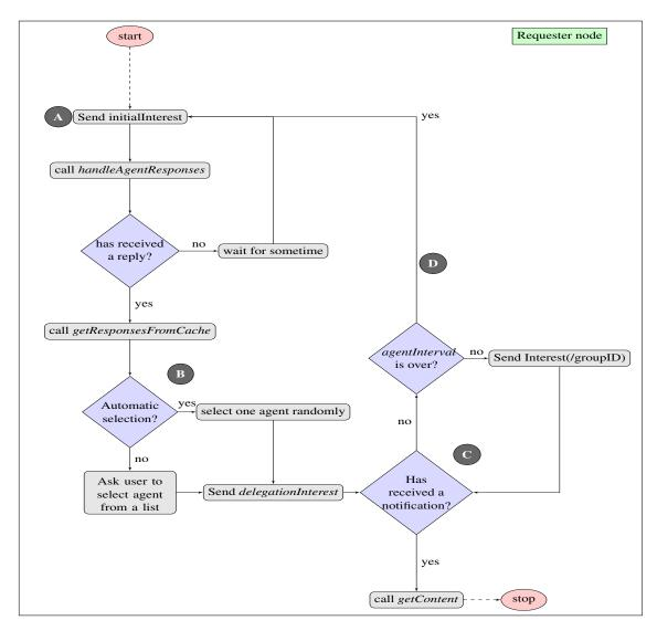
Figure 4.1: Flow chart of the delegation process in the requester node
