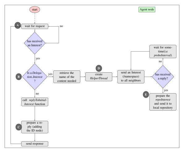
Figure 4.3: Flow chart of CCNAgent application tasks
