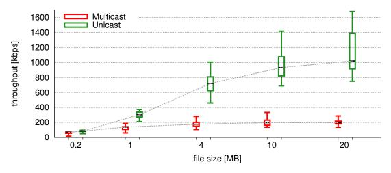
**Figure 5.4:** Throughput of the implemented mechanism tested with unicast and multicast communication between the agent and the content source.
