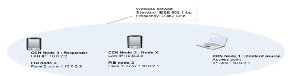
Figure 5.7: Topology used to evaluate congetfile application over two hops unicast communication.
