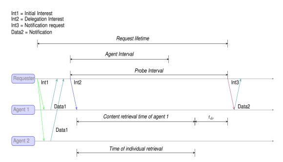
Figure 5.20: Messages exchanged during scenario 3: probe interval is higher than the agent interval
