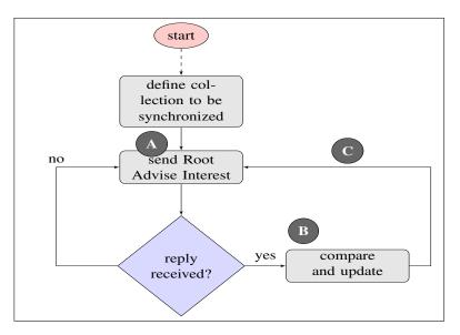
Figure 3.6: Flowchart of permanent synchronization
