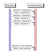
(a) Normal content retrieval using ccngetfile application over one hop
