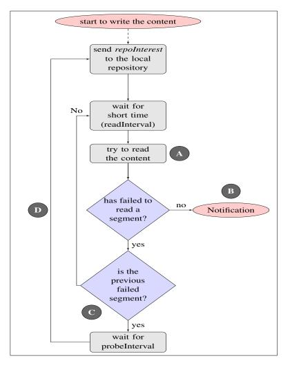
Figure 4.5: Flow chart of the verification mechanism in the agent node
