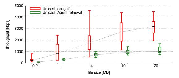
**Figure 5.8:** Throughput of the implemented mechanism compared with congetfile content downloads. The communication is performed via unicast according to the test setups.
