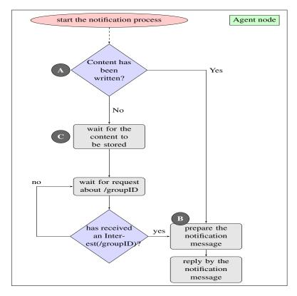
Figure 4.4: Flow chart of the notification process
