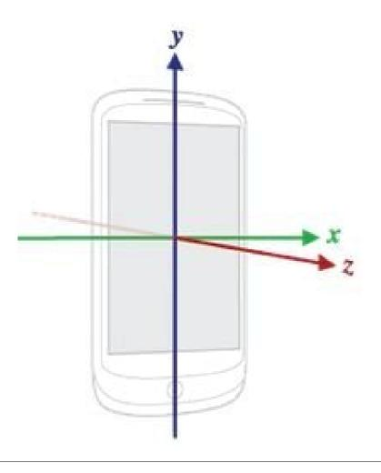
FIGURE 2.2: The values in the device's coordinate system.
