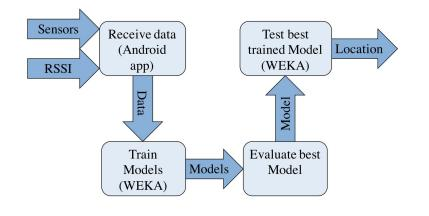
FIGURE 3.1: The architecture of the implemented android app.
