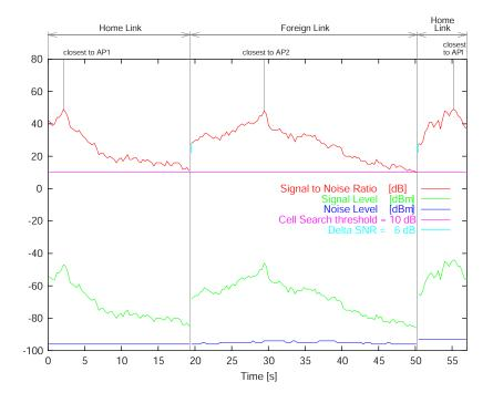
Figure 4.2: Signal to noise ratio when roaming with low AP density
