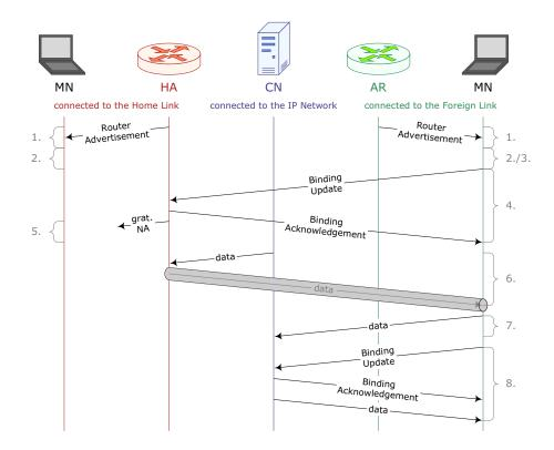
Figure 3.3: Mobile IPv6 operation Time-Message-Diagram
