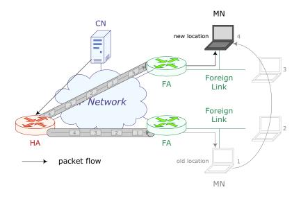
Figure 5.2: Out-of-date location information causing packet loss
