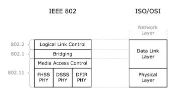
Figure 2.3: IEEE 802 layers vs. ISO/OSI Basic Reference Model
