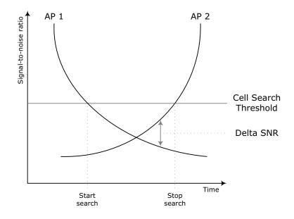
Figure 2.8: Link layer handover SNR-time diagram
