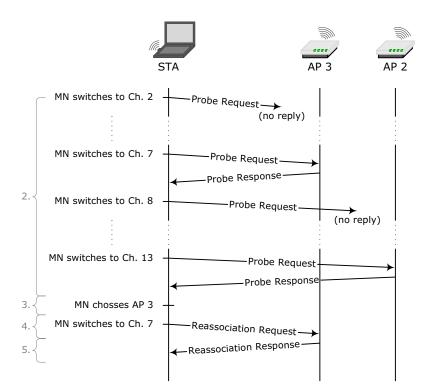
Figure 2.7: Link layer handover message-time diagram using active scanning
