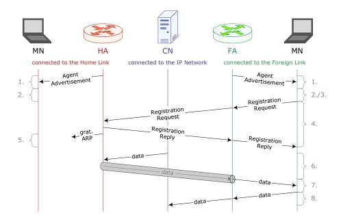
Figure 3.2: Mobile IPv4 operation Time-Message-Diagram
