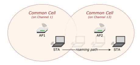
Figure 2.6: Roaming between two wireless cells
