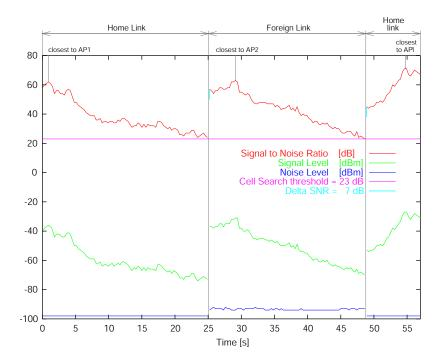
Figure 4.3: Signal to noise ratio when roaming with medium AP density
