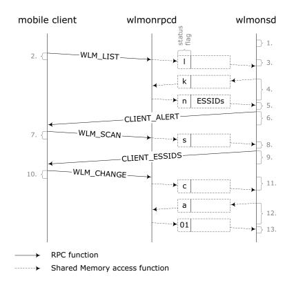
Figure 6.3: Wireless LAN Monitor procedure message-time diagram
