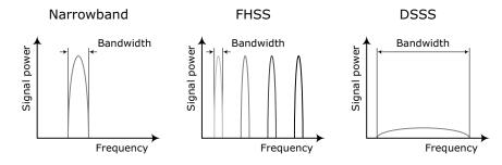
Figure 2.1: Transmitted energy distribution over frequency spectrum
