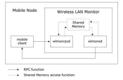
Figure 6.1: Interaction of the Wireless LAN Monitor components
