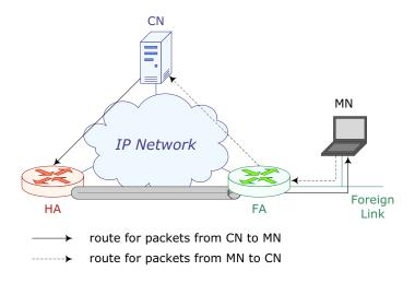
Figure 5.1: Sub-optimal triangle routing
