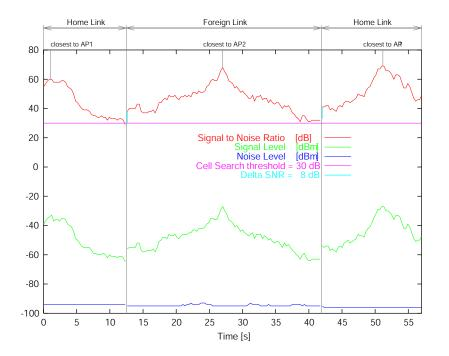
Figure 4.4: Signal to noise ratio when roaming with high AP density
