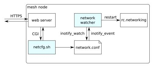
Figure 4.4: OViS remote network configuration.
