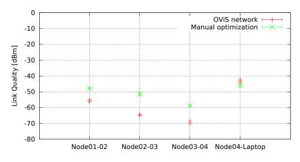
Figure 6.4: Manually improved link quality on OViS network (A).
