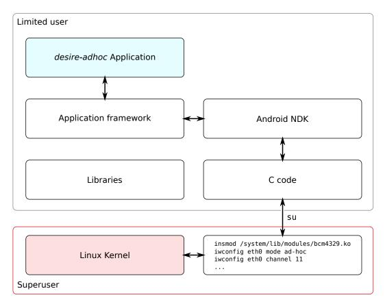
Figure 2.7: Root access through the Android NDK.
