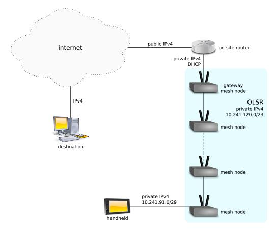
Figure 3.4: IPv4 Network topology.
