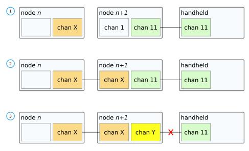
Figure 3.5: Deploying node n + 1.
