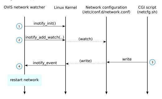
Figure 4.5: OViS remote network configuration.
