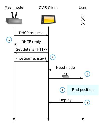
Figure 3.8: Network deployment with DHCP (dismissed).
