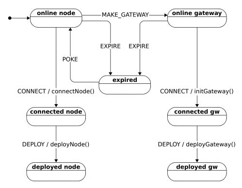
Figure 5.1: Node states as modelled in the OViS application.
