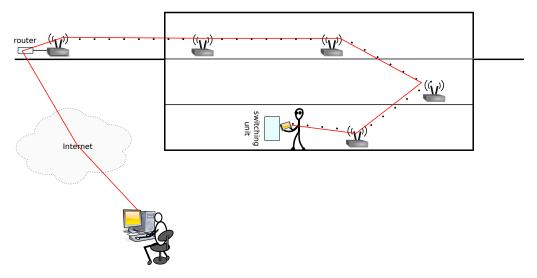
Figure 1.3: The solution: a wireless mesh network.
