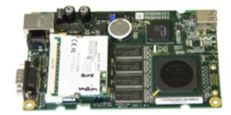
Figure 4.1: An OViS mesh node.
