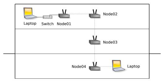
Figure 6.2: OViS testbed setup.
