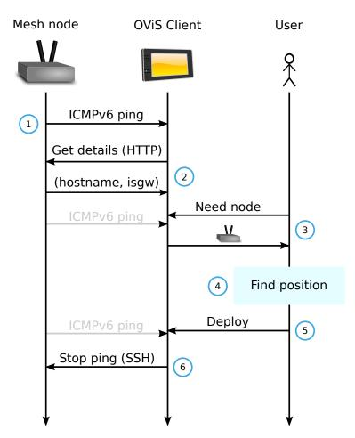
Figure 3.9: Network deployment with IPv6 auto-configuration (dismissed).
