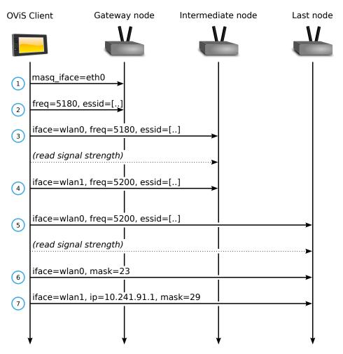
Figure 4.3: Typical sequences of network configuration commands.
