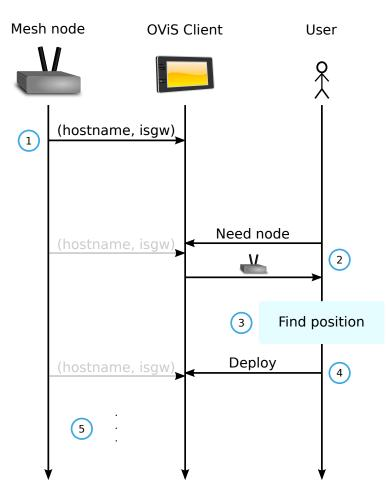
Figure 3.10: Network deployment with UDP pinger (accepted).
