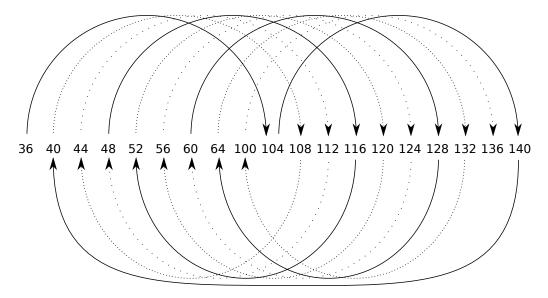
Figure 3.6: IEEE 802.11a channel allocation in OViS.
