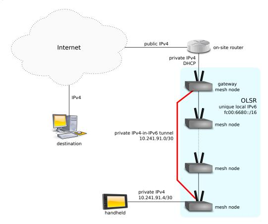
Figure 3.2: Network topology with an IPv4-in-IPv6 tunnel.
