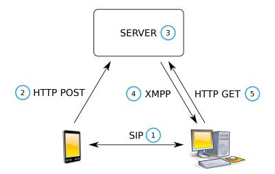
Figure 5.9: Communications using the OViS Android application.
