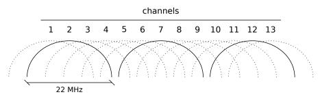
Figure 2.4: Overlapping frequencies in IEEE 802.11b.
