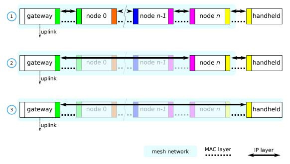
Figure 2.2: IEEE 802.11s mesh networking compared to OLSR.
