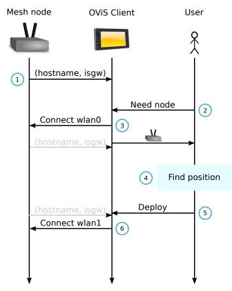
Figure 3.11: Final network deployment process, including mechanisms for multi-channel networking.
