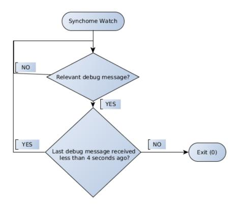
Figure 3.4: Syncwatch Flow
