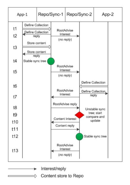
Figure 2.5: Illustration of the Synchronization Protocol[4]
