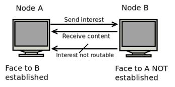
Figure 3.5: Impact of IP face registration on sync operation
