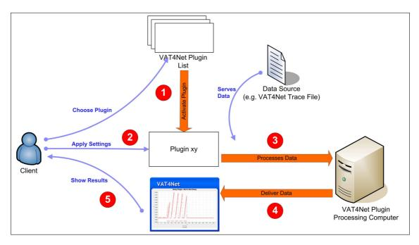
Figure 5.15: VAT4Net Plugin Architecture - workflow of the plugin engine.
