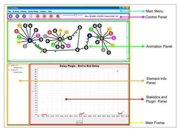
Figure 5.5: Overview of the application of GUI VAT4Net
