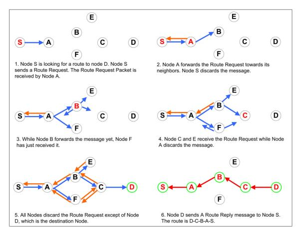
Figure 7.7: LAR Flooding Algorithm
