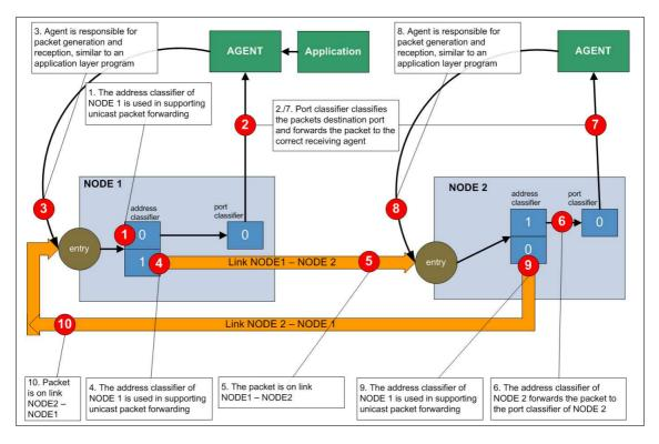
Figure 7.5: Packet Cycle on Node and Link in ns-2
