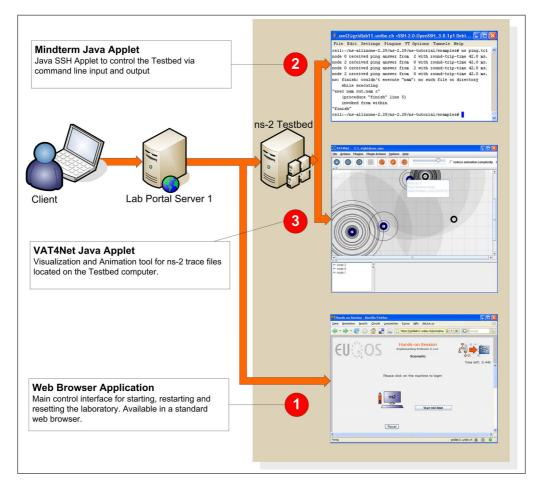
Figure 6.1: ns-2 Platform - showing the different interaction possibilities with the Platform.
