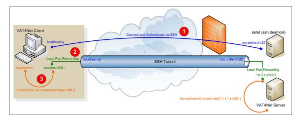
Figure 5.4: VAT4Net Connection setup with SSH Port Forwarding
