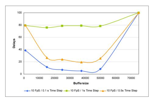
Figure 5.17: VAT4Net - Delay in subject to the buffer size
