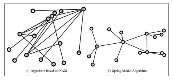
Figure 5.10: Node Placing Algorithms
