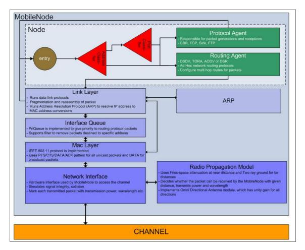
**Figure 7.6:** MobileNode Architecture
