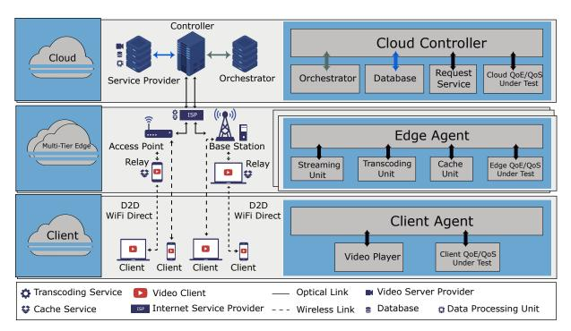
Figure 3: Multi-tier Edge Architecture for VoD Services. Source: [51]
