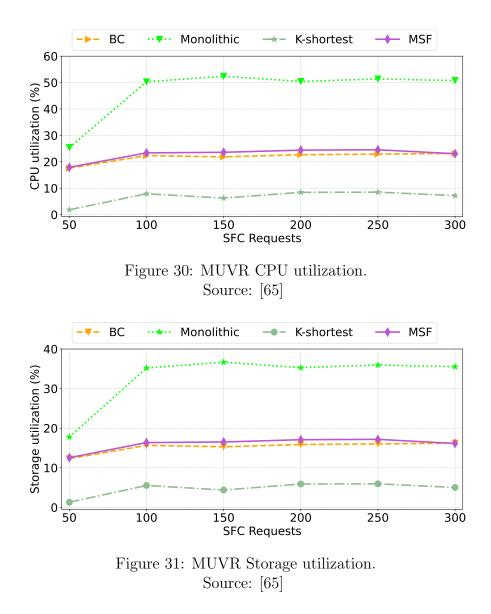
MSF shows more efficient network usage compared to BC for accepting fewer SFC requests and requiring more computational resources. K-shortest had smaller utilization for having a significantly lower acceptance ratio. MSF instantiates the SFs enabling the usage of edge nodes closer but bringing the SF instantiation to far away nodes, avoiding overloading the edge nodes and links.
