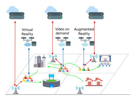
Figure 11: Multi-tier edge computing environment for mobile edge nodes and users. Source: author's own.
