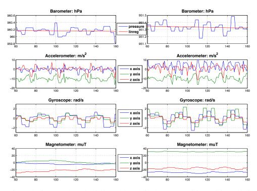
**Figure 5.1:** Graph of sensor values of activity 'walking' (left column) and activity 'walking an inclination up' (right column) in a 5 second window.
