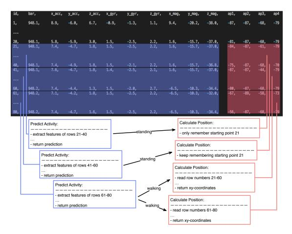
Figure 4.12: Adjustment of the time window while standing.
