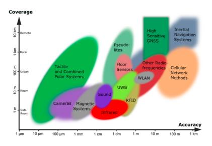
Figure 2.2: Overview of indoor positioning technologies in dependence on accuracy and coverage [2].
