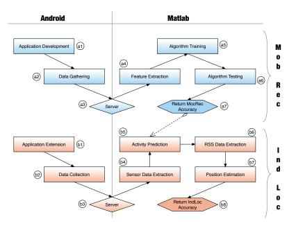
Figure 4.1: Overall structure (MobRec=mobility recognition / IndLoc=indoor localization).
