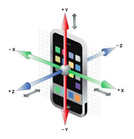
**Figure 2.1:** Embedded inertial sensors in smartphones measure a defined unit along three orthogonal axes, each splitted into a positive and negative part [27].
