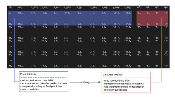
Figure 4.11: Adjustment of the time window while walking.
