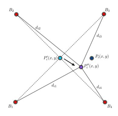
Figure 3.5: Exemplification of centroid and weighted centroid localization.
