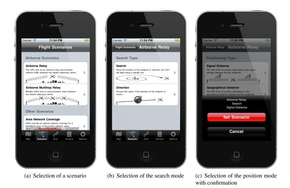
Figure 3.6: scenario view of the setup procedure for Airborne Relay on iPhone
