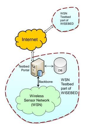
Figure 1: General testbed architecture. The figure shows the interconnection of wireless sensor testbeds via the Internet with the help of a Portal server. The Testbed Portal is connected with the testbed with a wired or wireless backbone.
