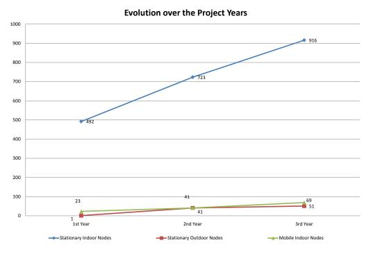
Figure 8: Evolution of number of wireless sensor nodes at partners. The graph shows the number of wireless sensor nodes over the tenure of WISEBED.
