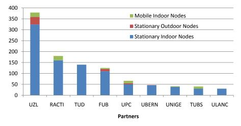
Figure 4: Number of nodes at partners. The graph shows the number stationary, mobile, and outdoor wireless sensor nodes.
