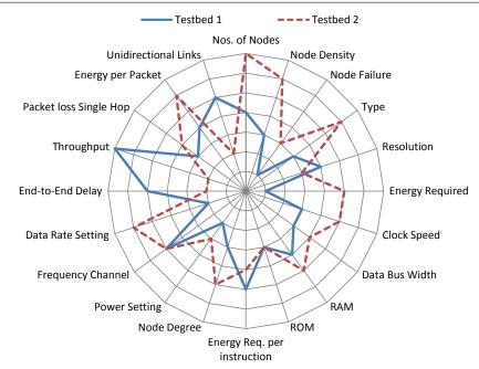
Figure 9: Benchmarking of different testbeds. The strengths and weaknesses of both WSN testbeds are visible from the different values of performance metrics.
