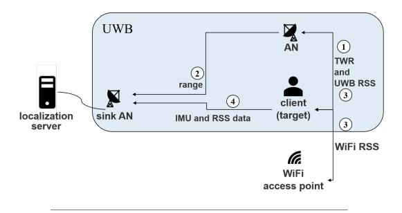
FIGURE 3.1: Overview of the components in our localization system.
