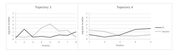
FIGURE 5.6: Measured distance errors at each checkpoint in trajectory 3 and 4.
