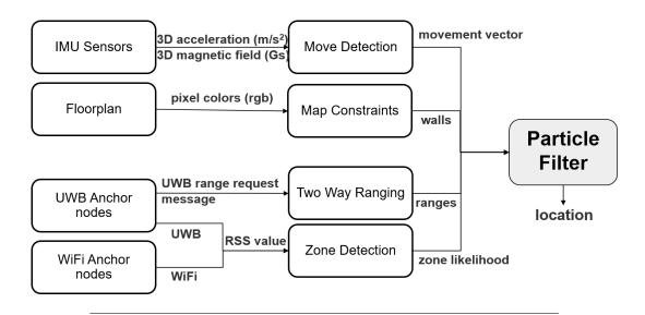
FIGURE 3.2: Overview of the localization algorithm components.
