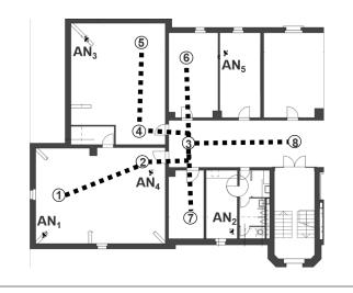
FIGURE 5.2: Trajectory 5 with improved anchor positions.
