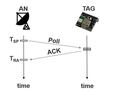
FIGURE 4.1: Minimal implementation of Two Way Ranging.
