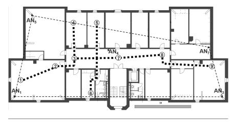
FIGURE 5.10: Indicated bounding box of the anchor node positions for trajectory 1.
