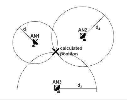
FIGURE 2.3: Graphical illustration of the trilateration concept.
