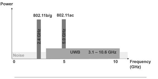
FIGURE 2.4: Comparison of Wi-Fi (802.11) and UWB frequencies.
