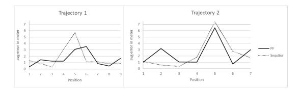
FIGURE 5.5: Measured distance errors at each checkpoint in trajectory 1 and 2.
