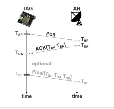
FIGURE 2.1: Illustration of TWR and SDS-TWR communication
