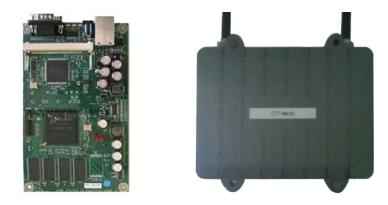
Figure 1.4: PC Engines WRAP node hardware with outdoor case
