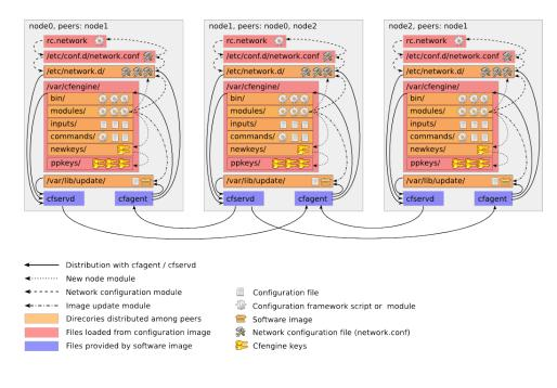
Figure 6.3: Configuration distribution with cfagent and cfservd.
