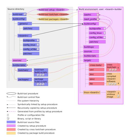
Figure 4.2: Details of the software build process
