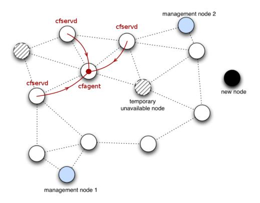
Figure 6.1: Interaction of cfagent and cfservd
