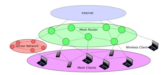
Figure 1.1: Example of a hybrid Wireless Mesh Network
