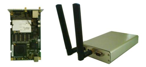
Figure 1.3: PC Engines Alix node hardware with indoor case
