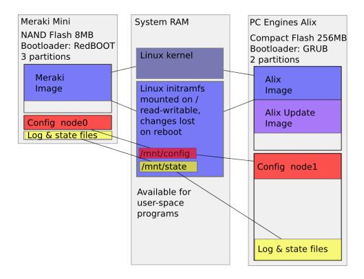
Figure 5.2: Run time layout of RAM and secondary storage of two platforms
