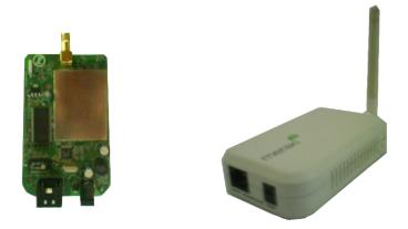
Figure 1.2: Meraki Mini node hardware with indoor case
