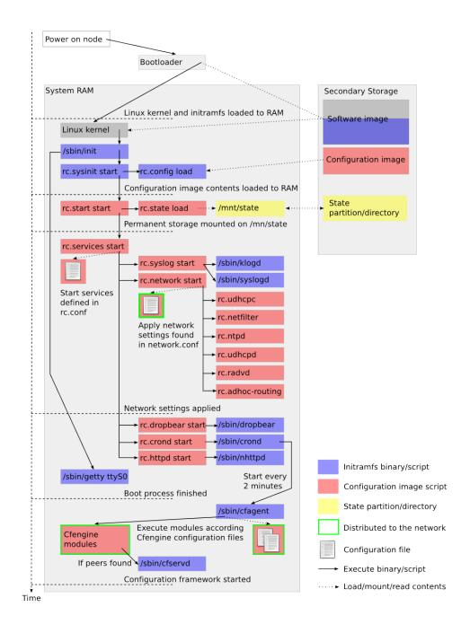
Figure 5.3: Details of the boot process
