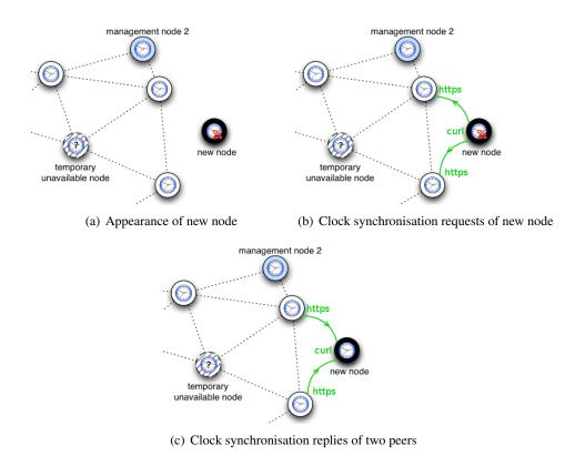
Figure 6.2: Synchronising system clocks between nodes
