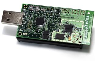
(a) Node with attached AA battery pack
