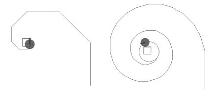
**Figure 23-12.** *Finding food by comparing distances and simply turning. Left: turn 45 degrees. Right: turn 15 degrees.*
