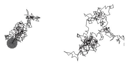
Figure 23-3. Walking with random angles of maximum 180 (left) and 360 (right) degrees
