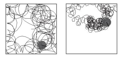
**Figure 23-6.** *Left: The insect moves in the opposite direction when confronted by a wall. Right: The insect chooses a random direction when confronted by a wall. This picture was obtained by setting the maximum length of the random walk to 10 pixels and turning a maximum of 90 degrees. To escape, it will make a random turn of a maximum of 360 degrees.*
