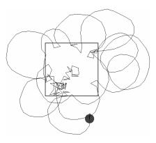
**Figure 23-9.** Second strategy. The bacterium increases the range of its directional change in a healthy environment. Here the speed is 25, and the change in direction is at most 36 in an unhealthy environment, and 360 in a healthy one.
