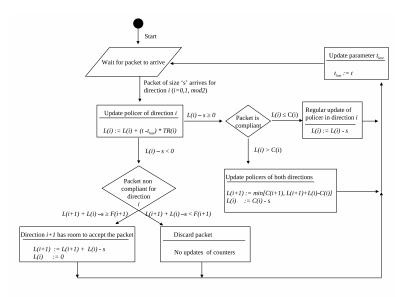
Fig. 1: State diagram for policing in two directions concurrently and preventing starvation in one of the directions. Here the parameters L(i), C(i), F(i), TR(i) denote respectively the bucket level, the ceil bucket limit, the floor bucket limit, and the token rate in direction i (i = 0,1, mod 2).
