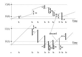
Fig. 2: Example of how the mechanism that polices traffic in the upstream and downstream directions concurrently. Index i = 0 denotes the upstream direction, with corresponding C(0) and F(0) as the ceil and floor limits. Index i = 1 denotes the downstream direction.
