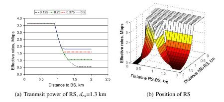
**Fig. 4.** Impact of RS characteristics on MS performance with SOBO scheduler: (a) RS transmit power; (b) RS position.
