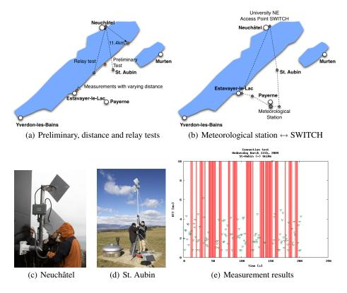
Fig. 1. Test scenarios and results of preliminary measurements Neuchâtel ↔ St. Aubin
