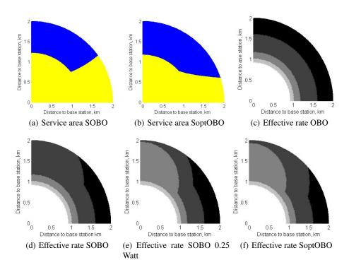
**Fig. 5.** Spatial behaviour in the cell with a relay station located at 1 km and transmit power 0.125 Watt. Shape of service area for: (a) SOBO and (b) SoptOBO. Effective data rates for: (c) OBO; (d) SOBO; (e) SOBO with RS transmit power 0.25 Watt; and (f) SoptOBO.
