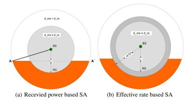
**Fig. 2.** Service area (SA) of a single relay station based on: (a) received power leves; and (b) effective data rates.
